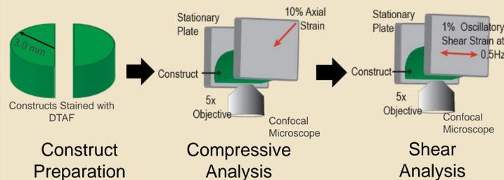
Digital image correlation (DIC) code analyzed movement and calculated strain<sup>8</sup>
